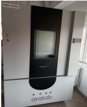
**Fig.1.** Equipment for temperature cycling test / Low temperature conditioning / High temperature conditioning
