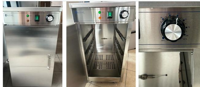
**Fig.10.** Equipment for High temperature conditioning test
