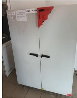
**Fig.2.** Equipment for temperature cycling test / High temperature conditioning
