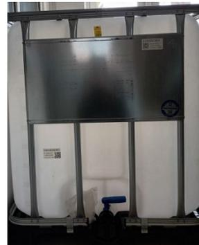
**Fig.6.** Vessel for the 24-hour immersion test
