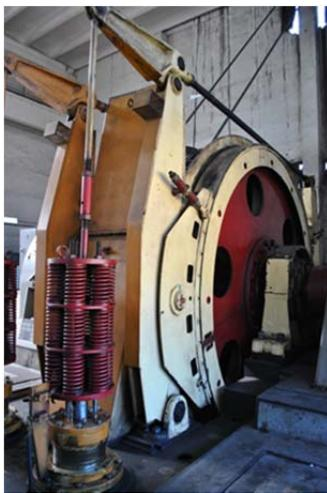
**Fig.2** Drive wheel and drum braking system from a mine hoisting machine
