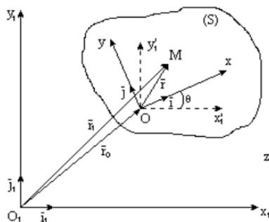
**Fig. 1.**  $S$  section in plane motion
