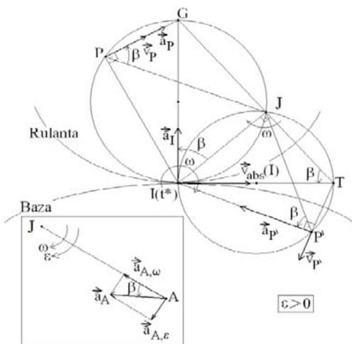
**Fig. 4.** Agreeing that  $\beta > 0$  if  $\vec{a}_A$  is on the right of the  $JA$  segment
