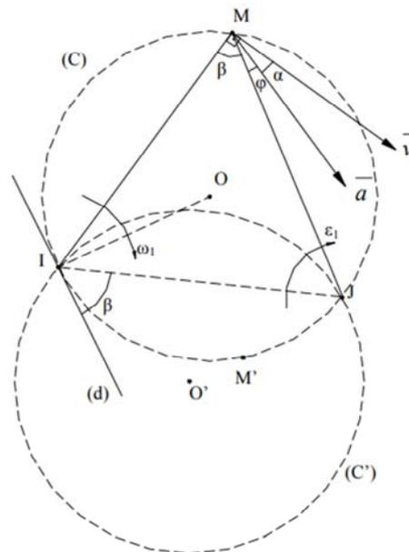
Fig. 2. Graphic construction of isocline circles
