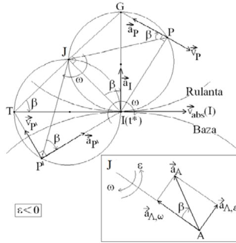
**Fig. 5.** Agreeing that  $\beta < 0$  if  $\vec{a}_A$  is on the left of the  $JA$  segment
