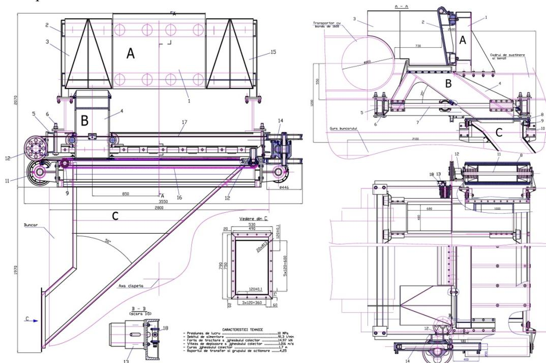
Figure 1. Automatic installation for taking elementary samples of lignite
