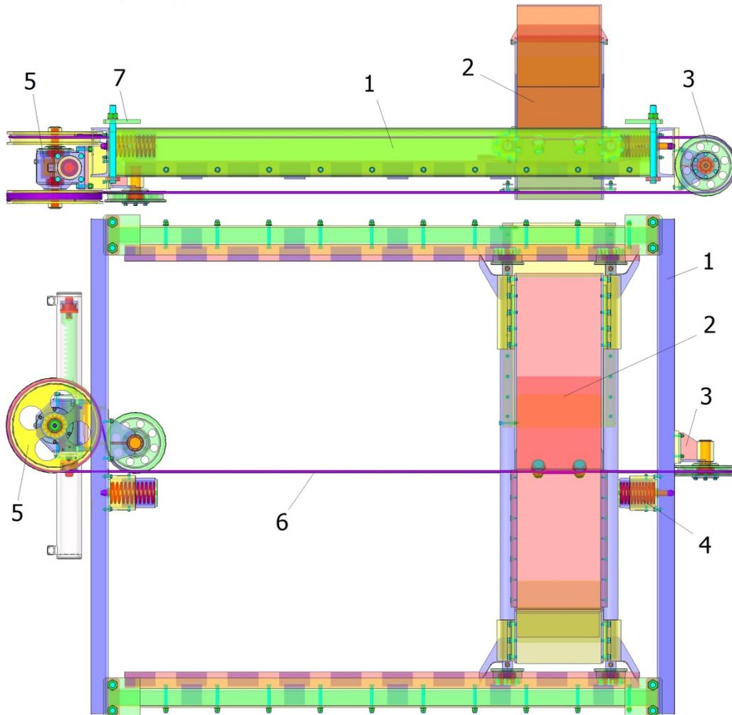
**Figure 2.** Device for taking the lignite sample from the discharge stream from the belt conveyor
