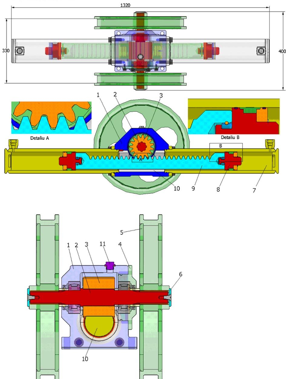
**Figure 4.** The 3D model of the drive group for the automatic plant to take samples of lignite from the stream to be loaded into wagons
