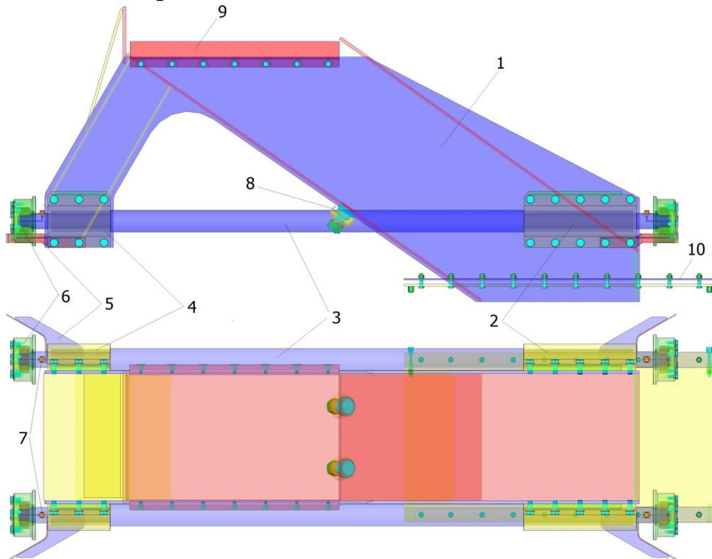
**Figure 3.** Chute for taking lignite samples
