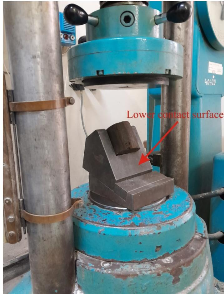
**Fig.1.** Hydraulic press prepared for rock shear testing
