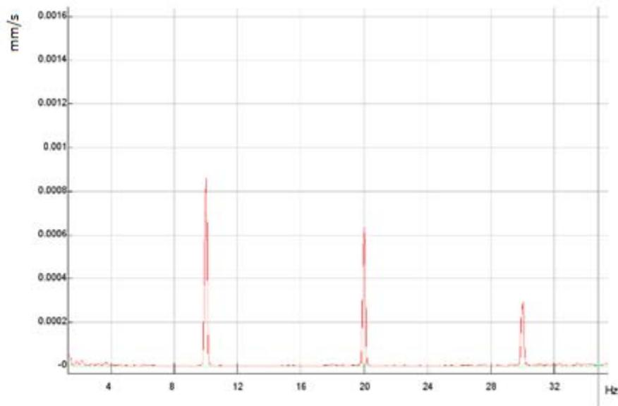
**Fig. 5.** Vibration FFT spectra on the fan
