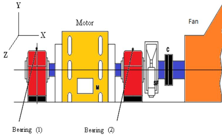
**Fig. 2.** Schema of the placement of the piezo accelerators
