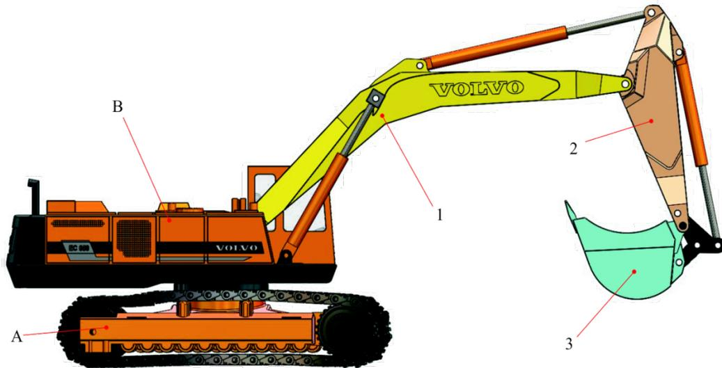
**Fig. 1.** Single bucket hydraulic excavator
