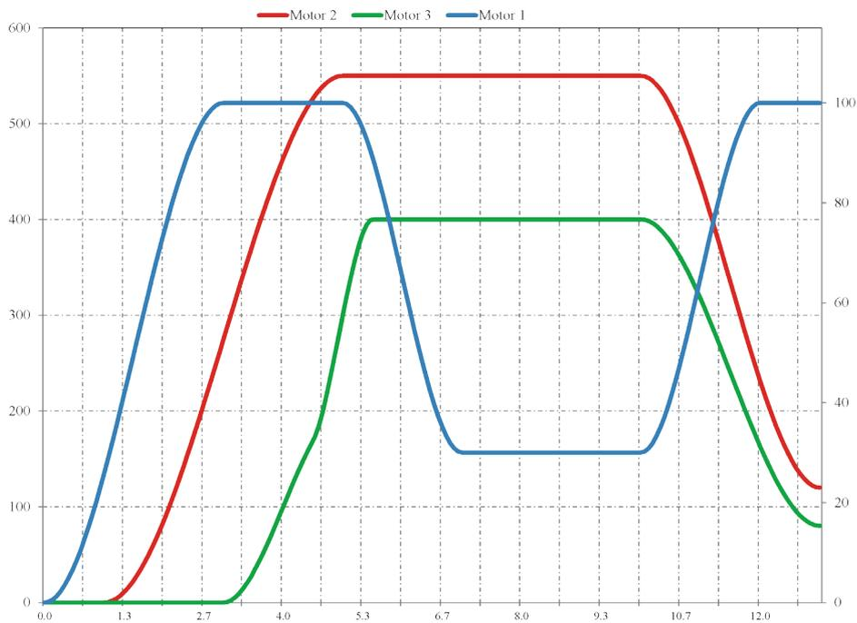
Fig. 5. Diagrams of the variation of the space travelled by each piston of the drive cylinders
