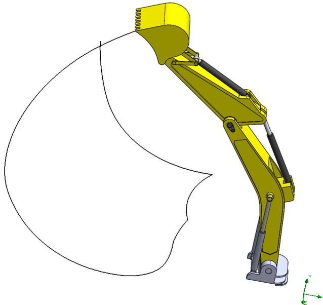
**Fig. 6.** The trajectory of a tooth from the bucket of the mini excavator
