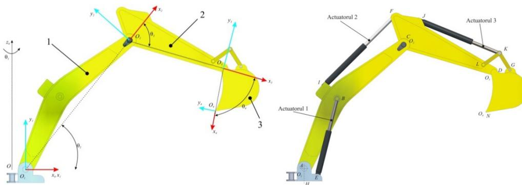
**Fig. 2.** Hydraulic excavator working equipment, coordinate systems attached to it and positions of hydraulic cylinders
