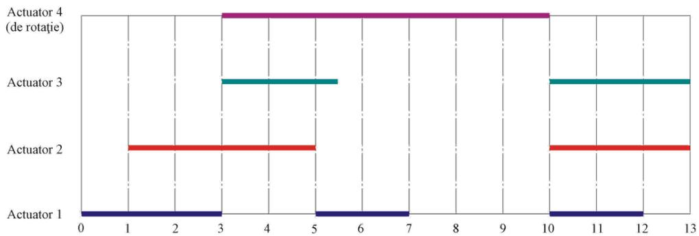
Fig. 4. Gantt chart highlighting the time sequence of the action of the four actuators
