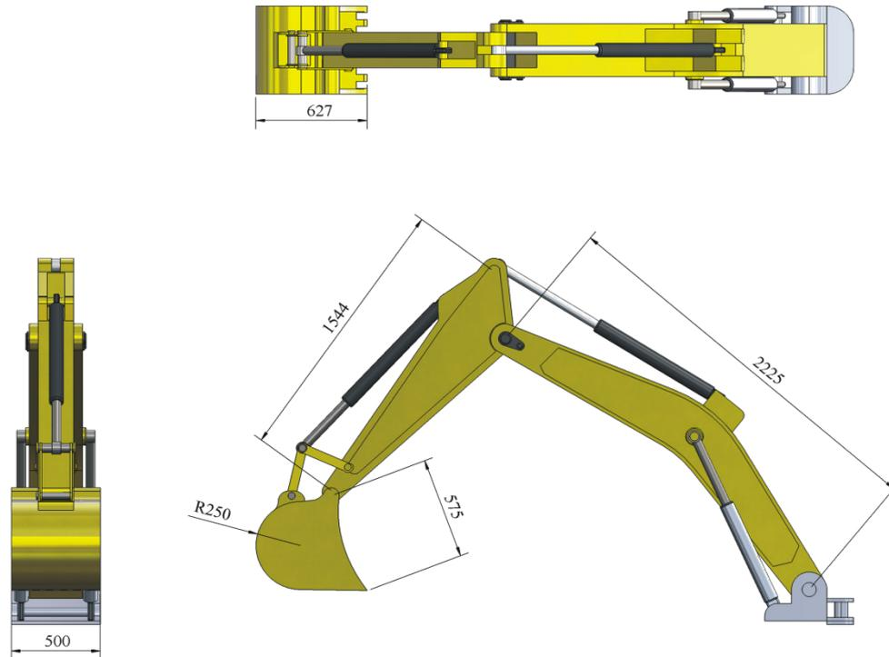
**Fig. 3.** Dimensions of the model of the excavator working equipment (in millimetres)
