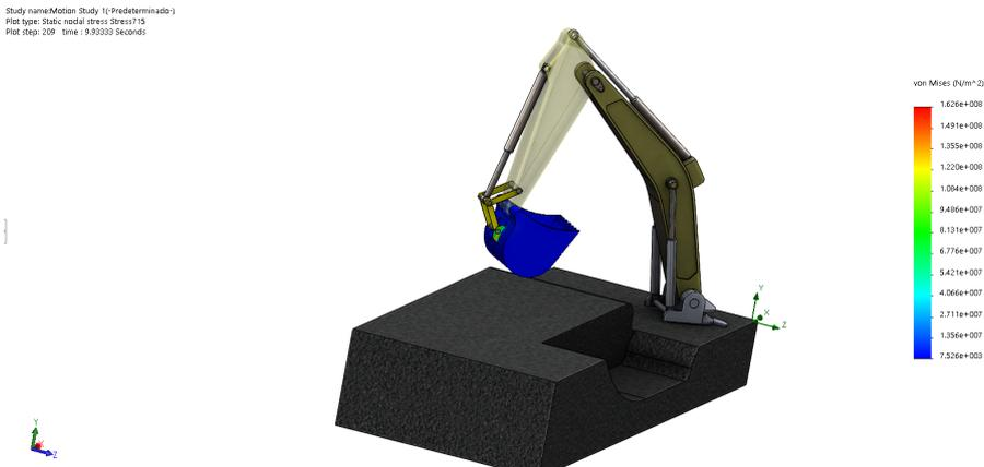
Fig. 11. Von Mises stress at the end of the excavator arm pivoting movement.
