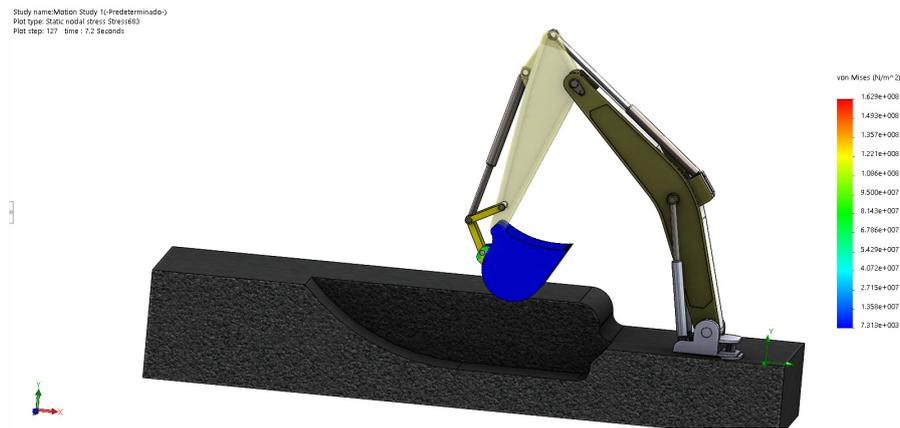
Fig. 10. Von Mises stress at the end of excavated material lifting
