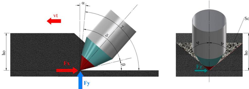
Fig. 2. Characteristics of cutting with conical picks
