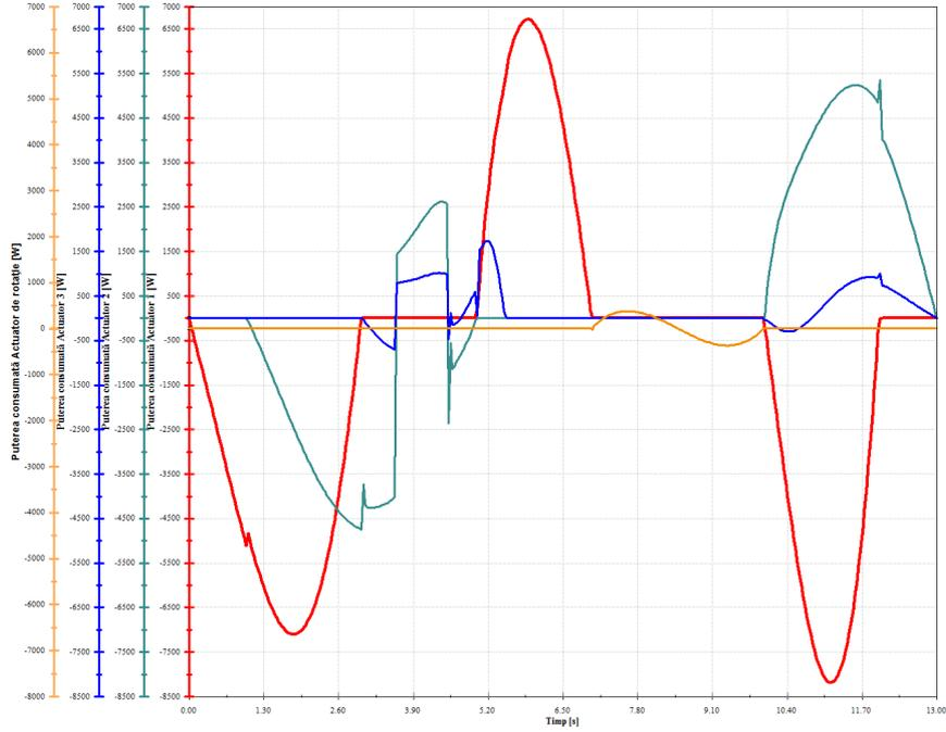
**Fig.6.** The variation of the driving power for each of the actuators during the simulation of the excavation process
