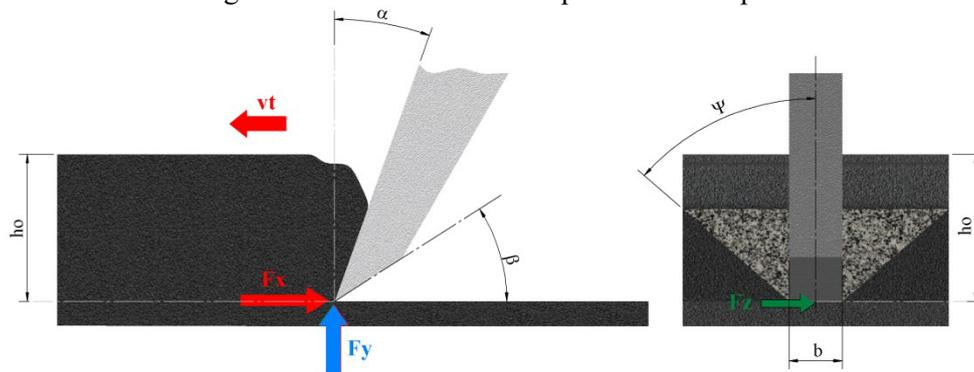
Fig. 2. Characteristics of cutting with chisel pick cutting tools
