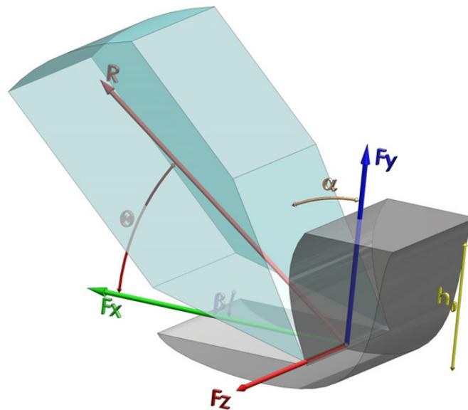
Fig. 1. Forces acting on the cutting tool
