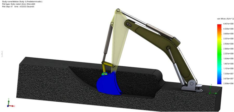
Fig. 9. Von Mises stress at the end of material cutting
