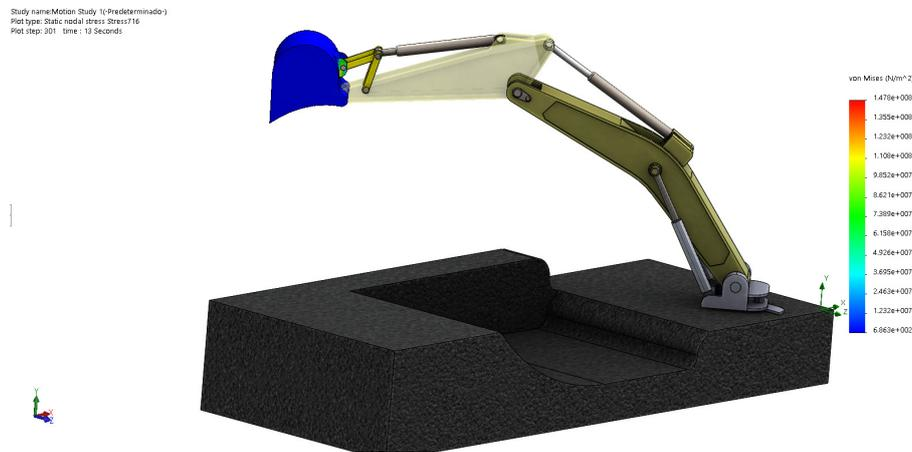
**Fig. 12.** Von Mises stress at the end of material discharge.
