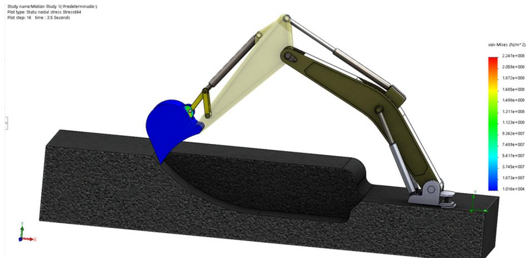
**Fig. 8.** Von Mises stress at the start of material cutting.
