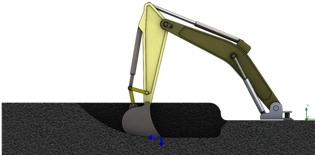
Fig. 4. Forces acting on the hydraulic excavator bucket
