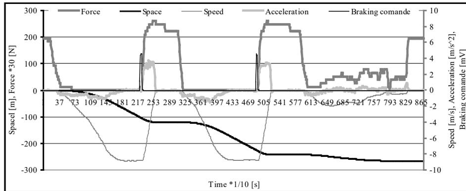
Fig.7. Right tie bar, left skip going down
