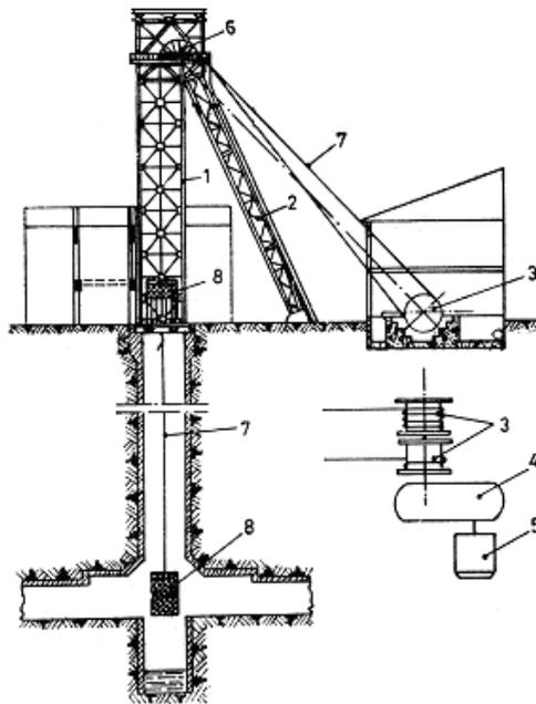
Fig.1. The principle draft of the extraction installation
