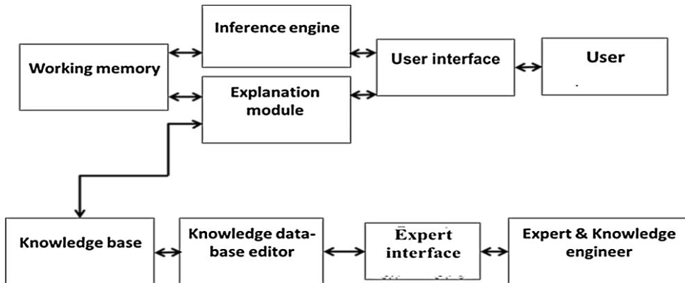
Fig. 3. Expert System components
