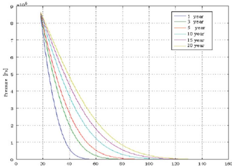
Fig. 7. Distribution of gas pressure along the damaged area near the interface[5]
