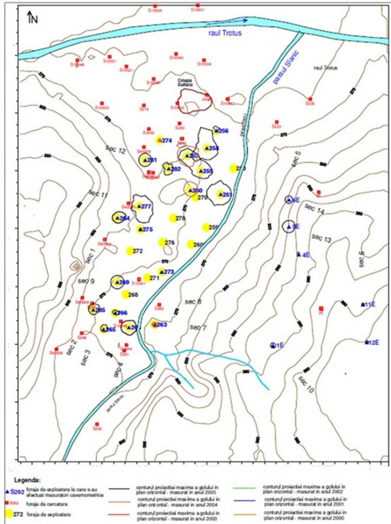
**Fig. 3.** Surface level curves, sections and boreholes positions at salt deposit Tg. Ocna [1]
