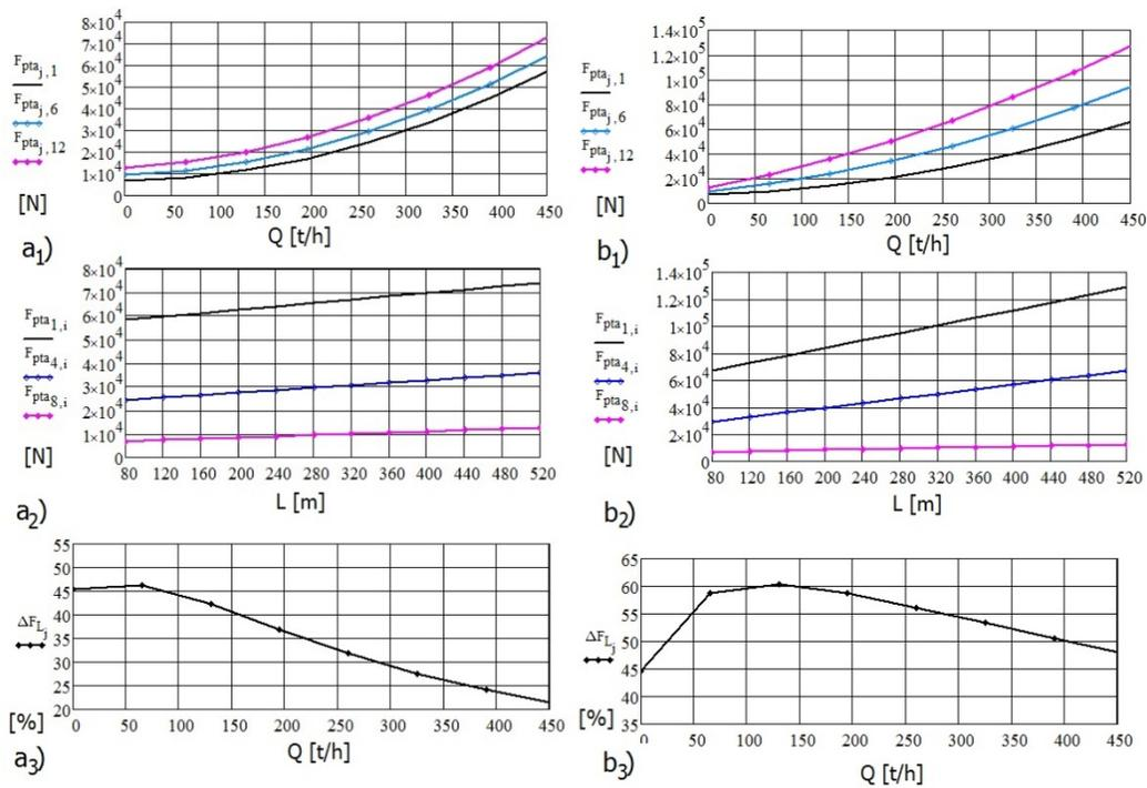
Figure 5. Variation of belt driving force function of the flow rate and length
