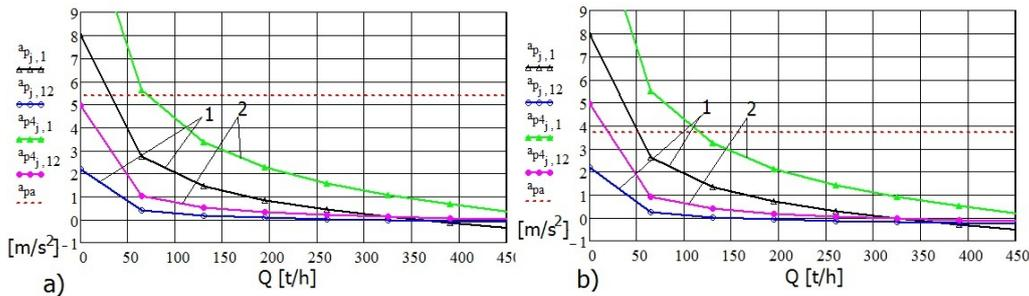
Figure 9. Starting accelerations variation depending on the belt sliding on the drum and on the coal sliding on the belt
