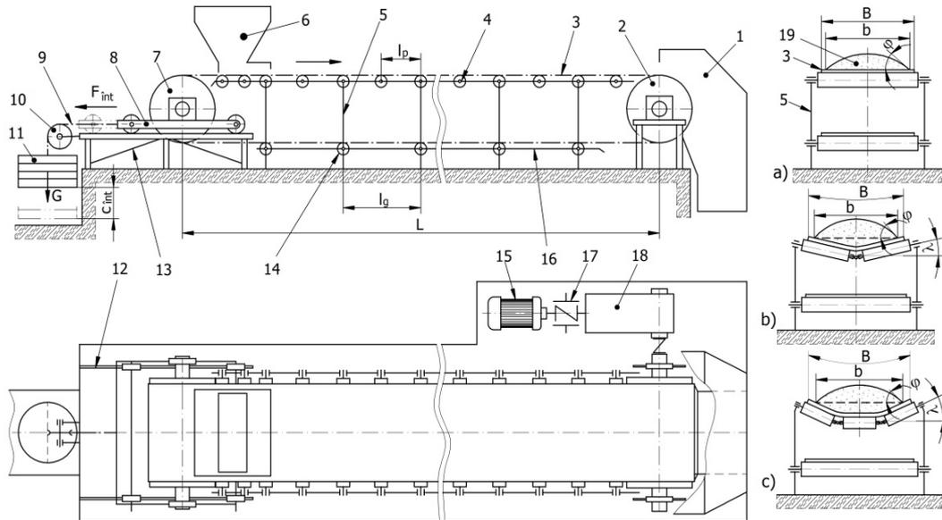
**Figure 1.** Construction diagram of a stationary roll belt conveyor
