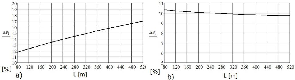
Figure 8. Percentage variation of power in idle run compared to the power for maximum capacity
