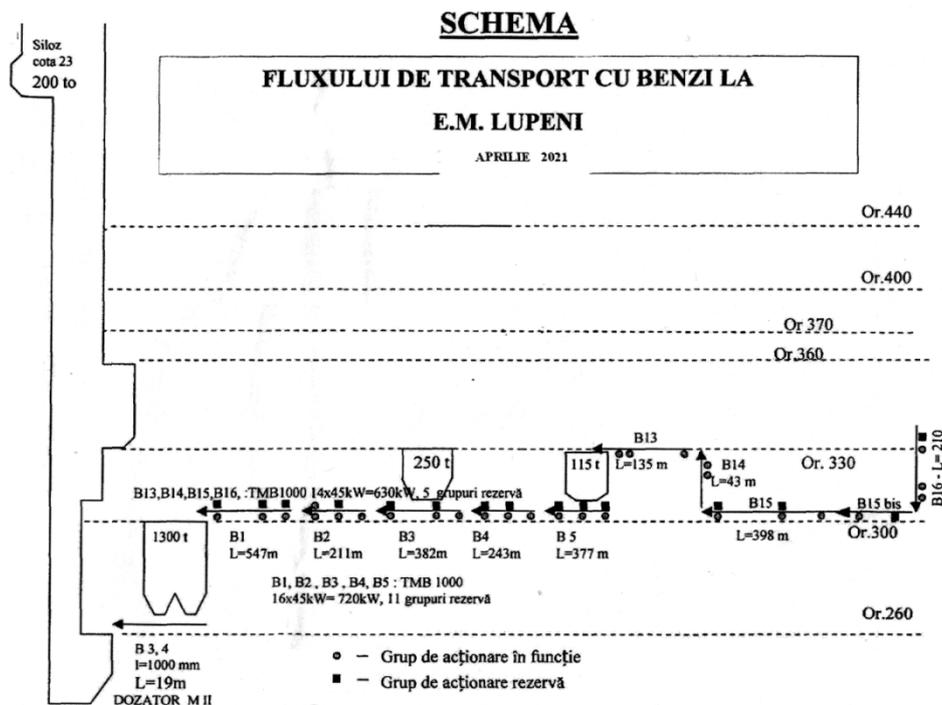
Figure 2. Diagram of haul flow with roll belt conveyers TMB1000-E.M.Lupeni
