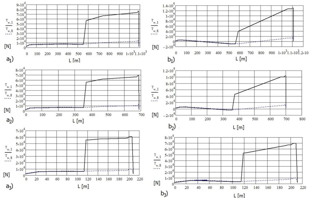
**Figure 4.** Graph of the traction forces in the conveyer belt
