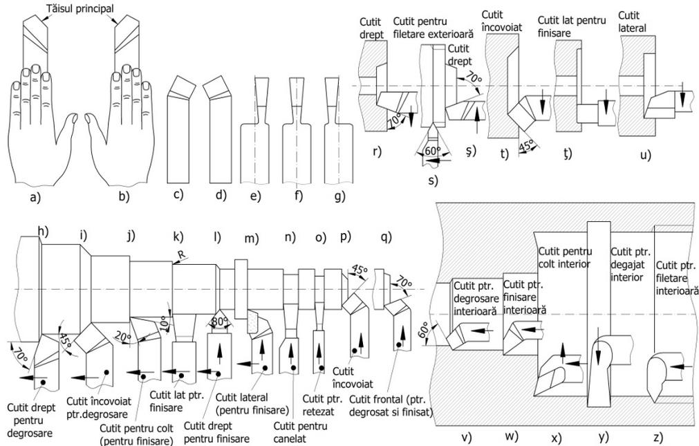
**Figure 1.** Constructive shape and processing by cutting of the lathe tools
