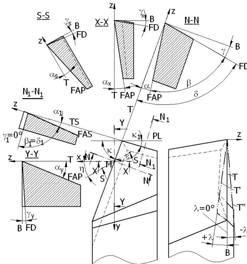
Figure 2. Constructive and functional angles of the lathe tool
