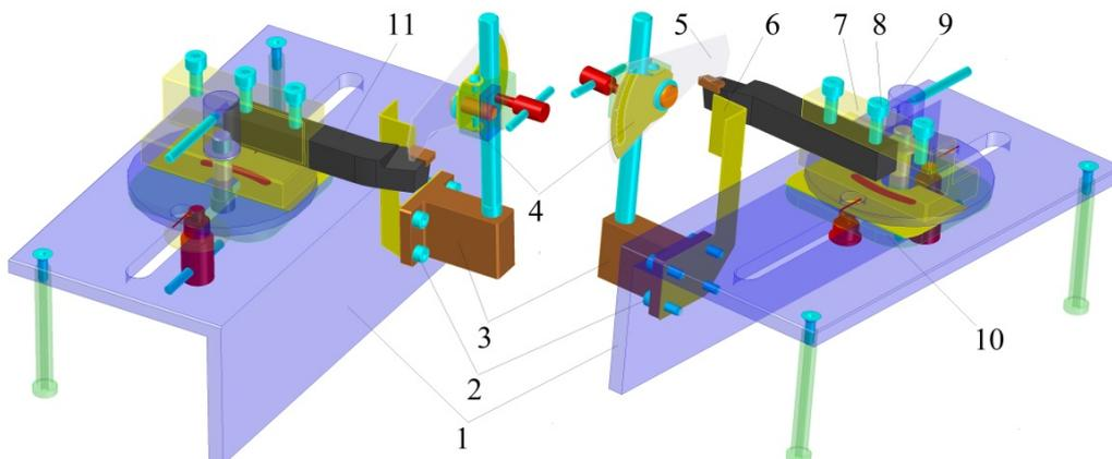
Figure 3. 3D model of the device for measuring lathe tool constructive angles
