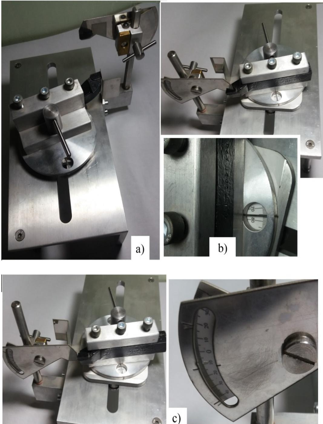
Figure 7. Measuring secondary angles of the lathe tool
