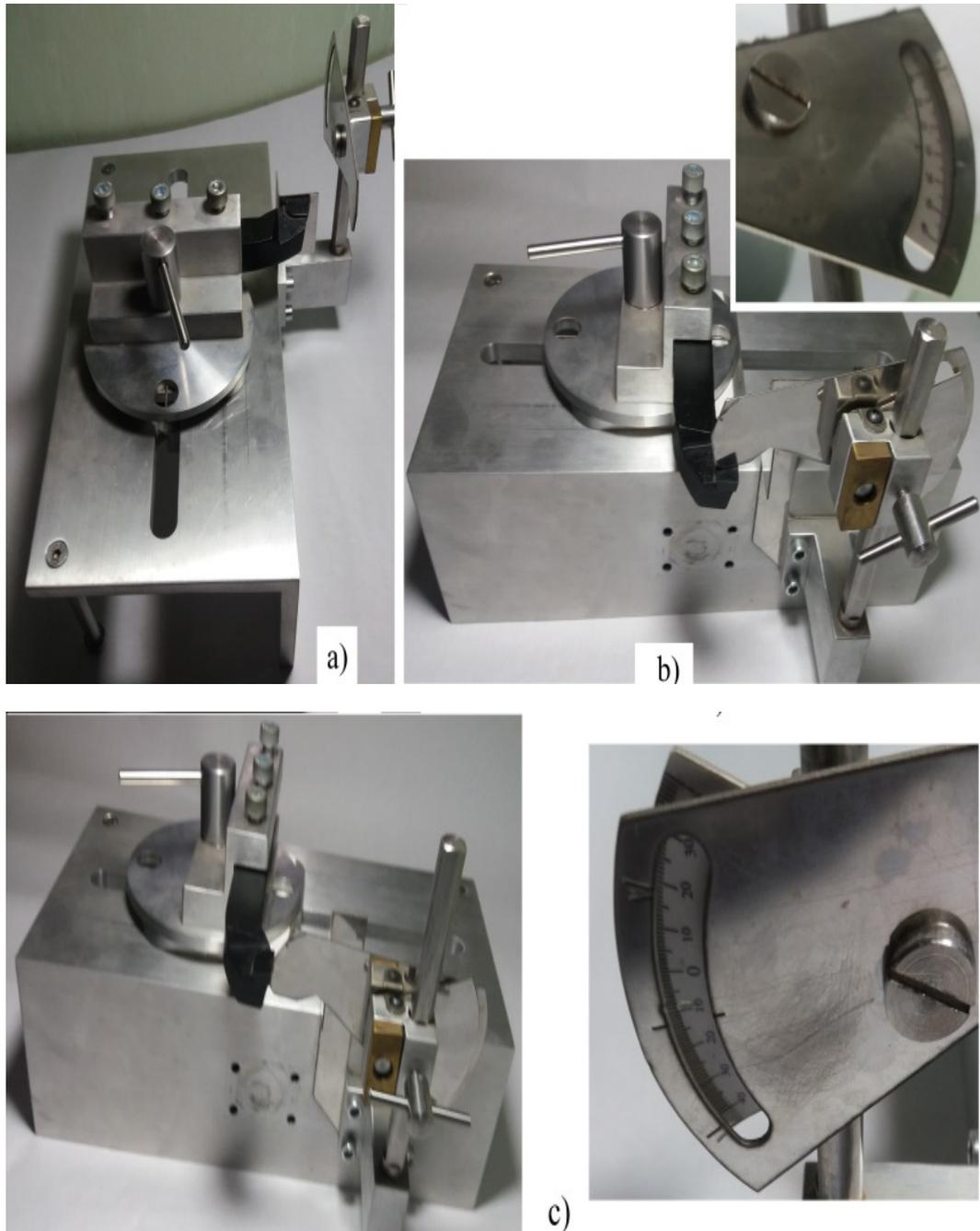
Figure 6. Measuring the main angles of the lathe tool
