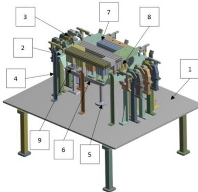
**Fig.1** Isometric view of the main components of the studied gluing station
