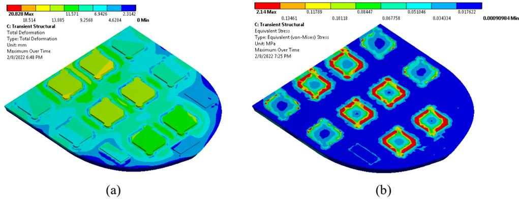
**Fig.3** Maximum over time total deformation (mm) and von-Mises Stress of the insulator
