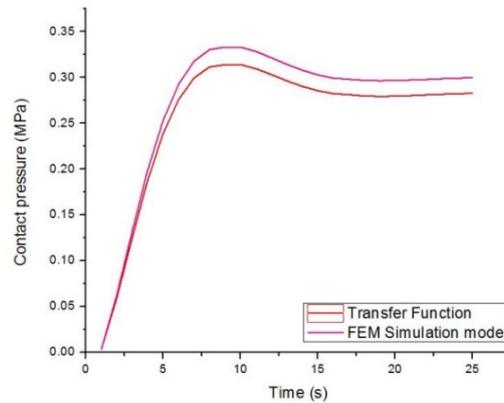
**Fig.4** Step response of the system achieved by the transfer function and FEM Simulation model
