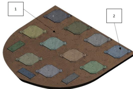
Fig.2 Simplified representation of insulator (1) and the piston-rod cushioning interaction area
