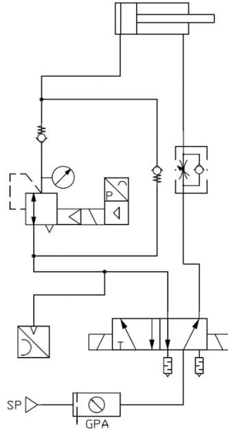
**Fig.2** Pneumatic diagram for the velocity and force control of a single cylinder
