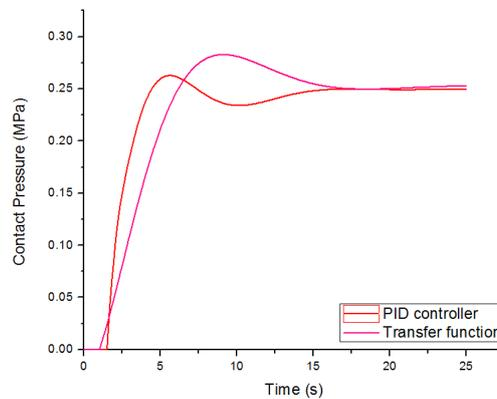
**Fig.5** Step response of the system achieved by the open-loop transfer function and the PID controller
