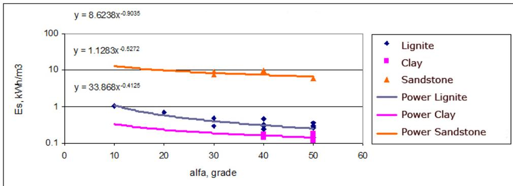
Fig. 2. Comparison upon  $W_S$  as function of  $\alpha$  (y log scale)
