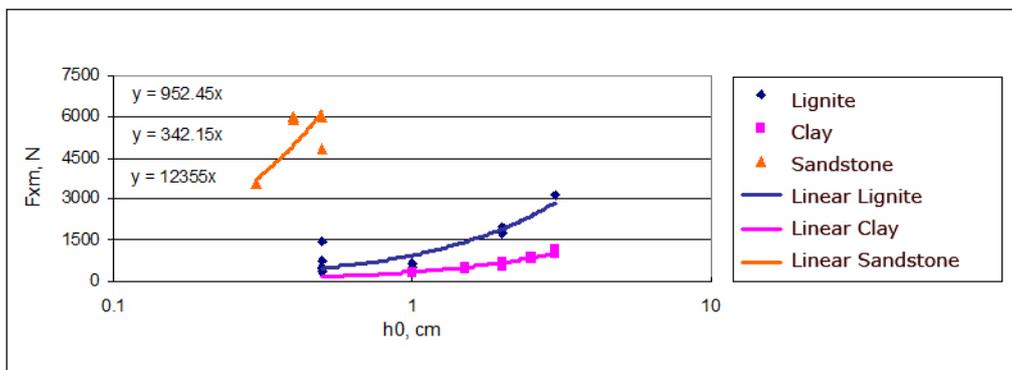
Fig. 1. Comparison upon  $F_{xm}$  as function of  $h_0$  (x log scale)
