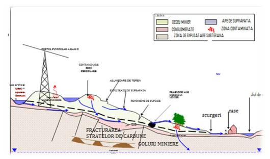
Fig. 6. Modelling of the flow of underground waters and of the transfer of contaminants within the analysed area (the perimeter of Lupeni)
