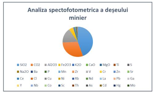
Fig. 7. Spectrophotometric analysis of the mining waste stored at Branch 1
