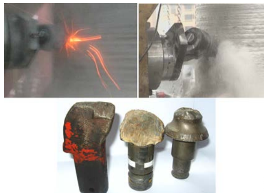
Fig.2 View of frictional sparking, dustiness during cutting of a rock sample with a rotary-tangential pick and wear of pick wedge
