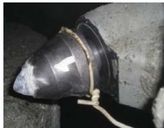
Fig. 9 View of the tool edge and holder surface after tests of rock sample cutting at the length of about 1000 m, with holder water feed
