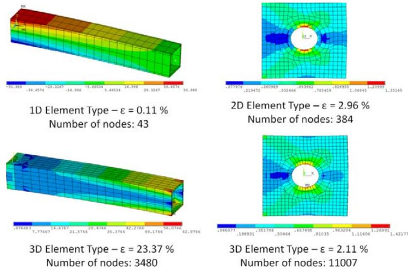
**Fig.2** Comparison of errors between 1D, 2D and 3D modeling approaches
