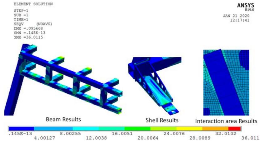
**Fig.4** Details of the Von-Misses stress distribution for beam, shell and interaction area results
