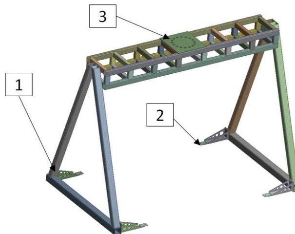
Fig.1 The geometric characteristics of a car-lifting end effector
