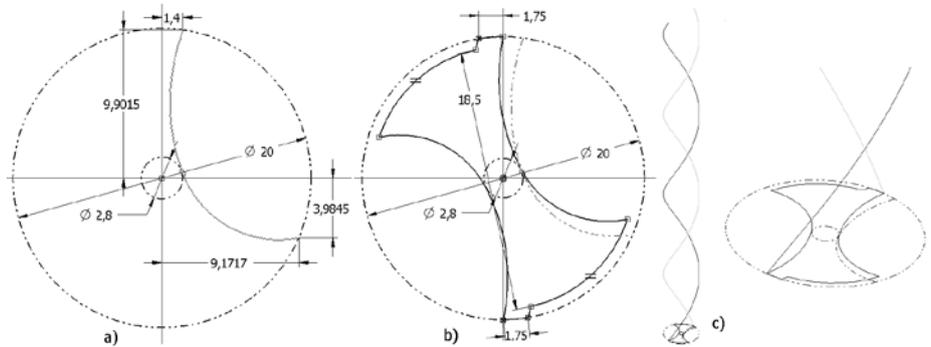
Fig. 3. The stages of carrying out the cross-section and of the steering curves of the drill
