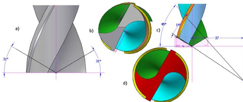
Fig. 6. The stages of 3D modelling of the settlement faces at the conical sharpening
