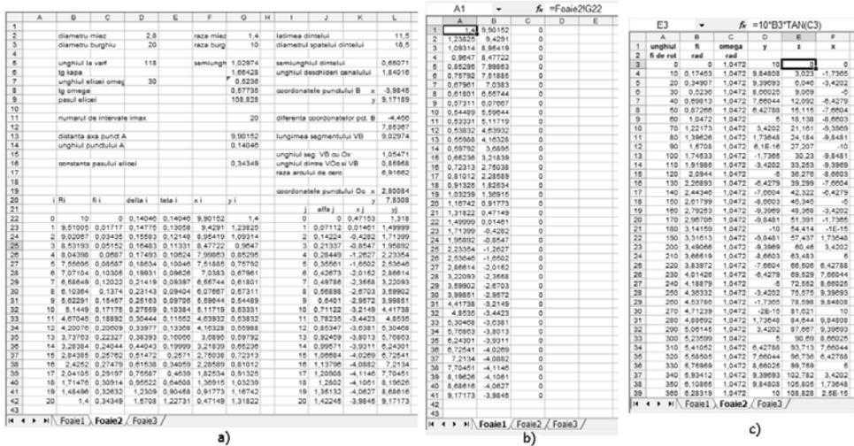
Fig. 2. Calculation of the helical channel profile in Excel
