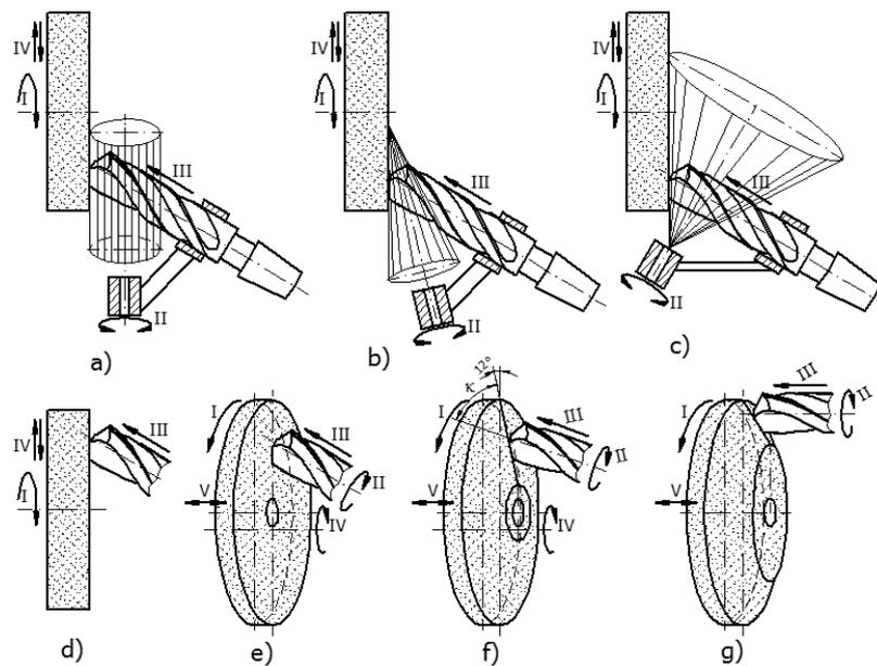
Fig. 5. Sharpening procedures
