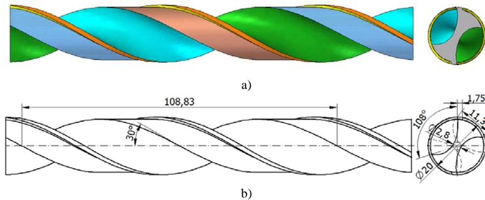
Fig. 4. The 3D model and the drawing of the active part of the helical drill
