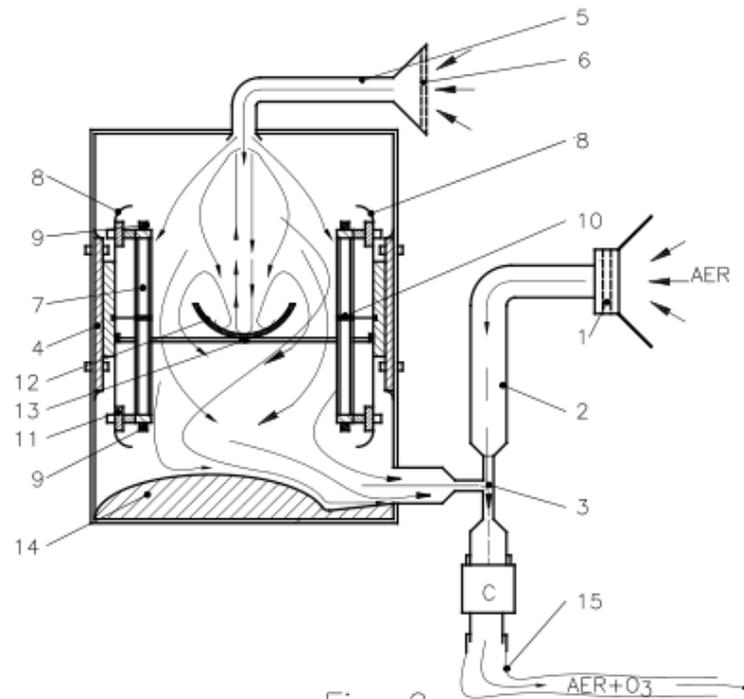
Fig. 2. Section through the ozone-generating device
