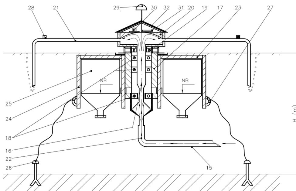
**Fig. 3.** Section through the ozonation device
