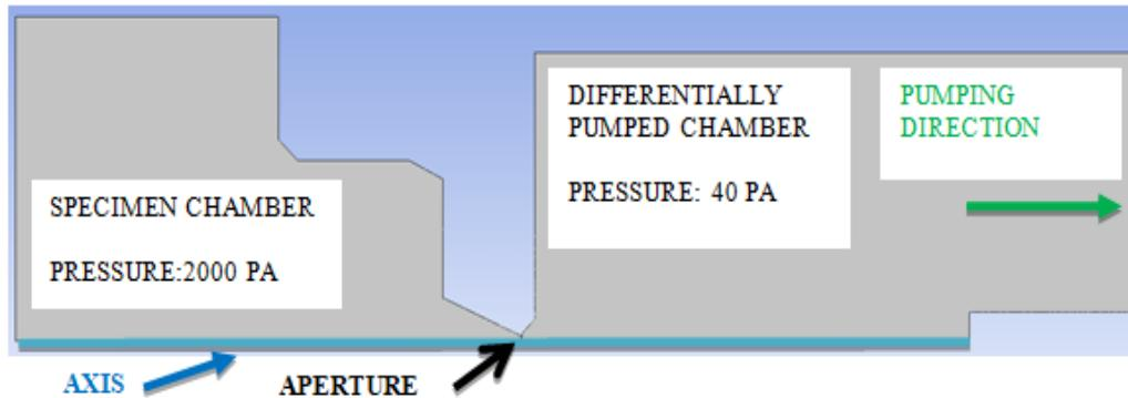
**Fig. 3.** Axisymmetric shape of the experimental chamber for simulations
