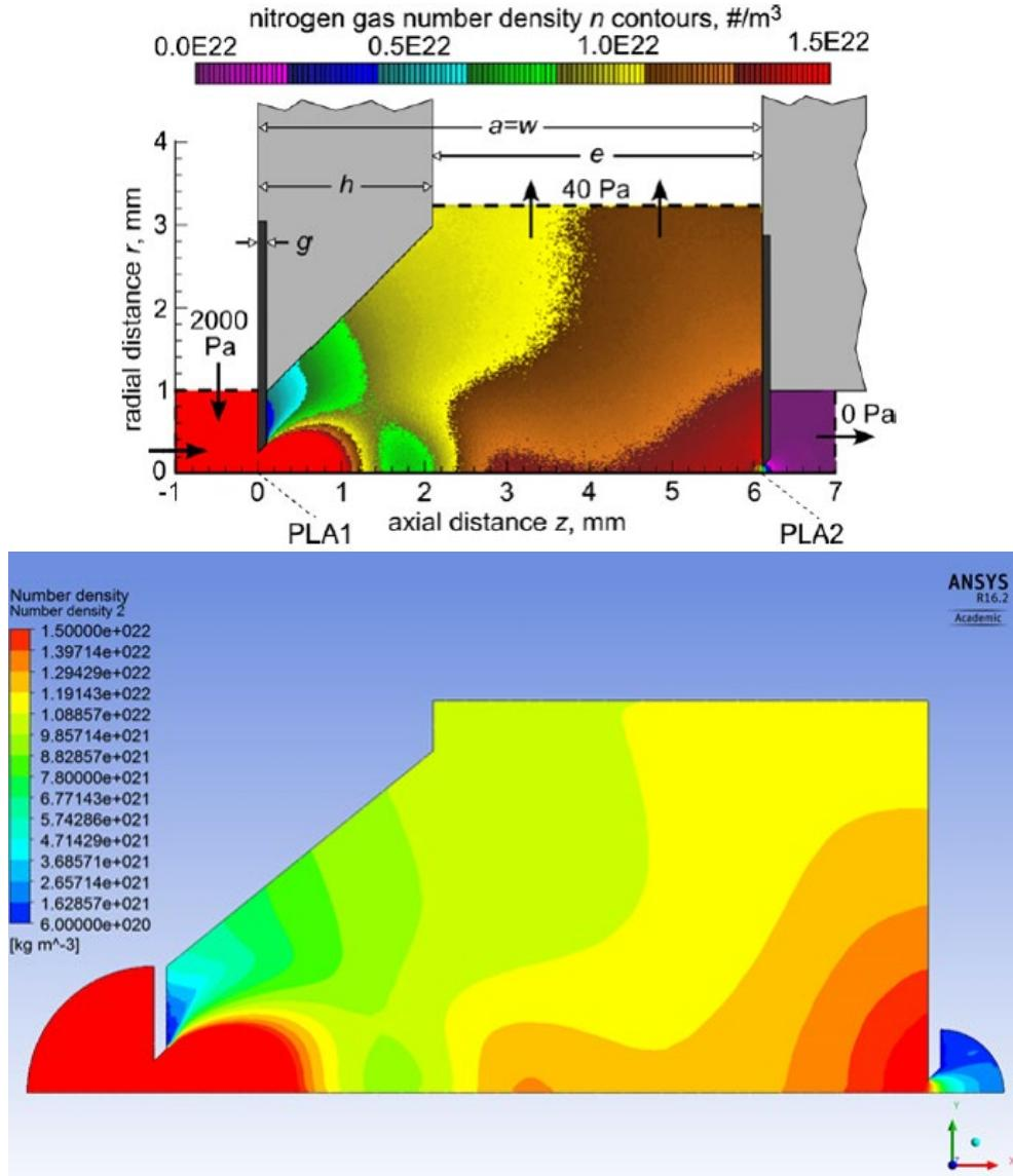
**Fig. 1.** Comparation of the analysis results obtained using Monte Carlo method and mechanism of continuum
