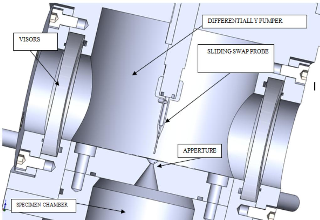
Fig. 2. Experimental chamber
