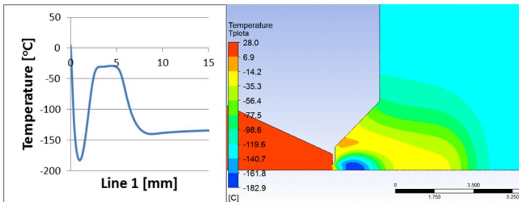
Fig. 7. Temperature layout above the aperture – line 1
