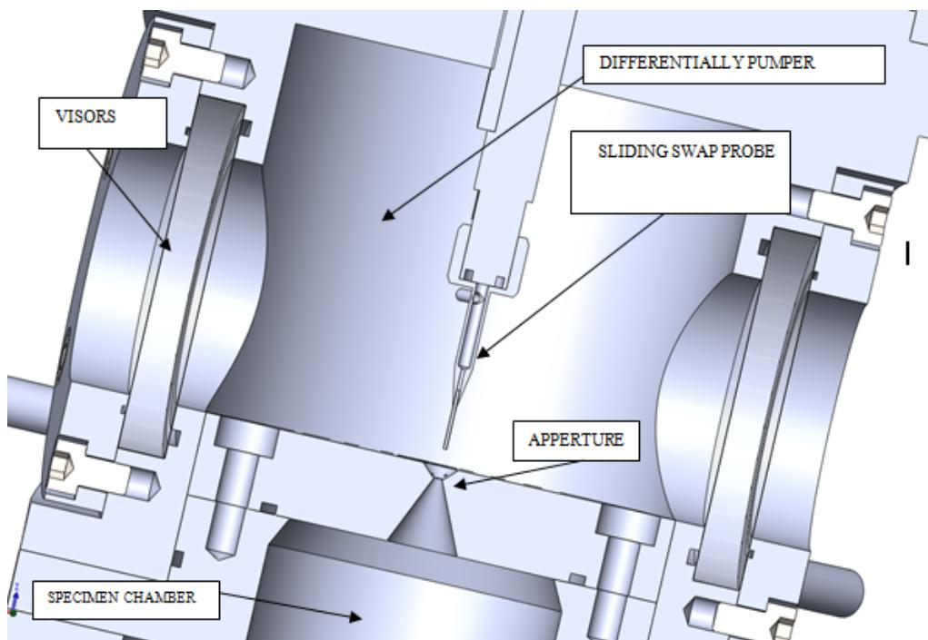
**Fig. 2.** Experimental chamber
