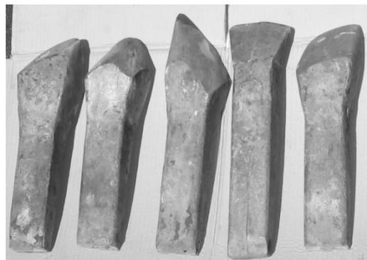
**Fig. 4.** Worn excavator teeth
