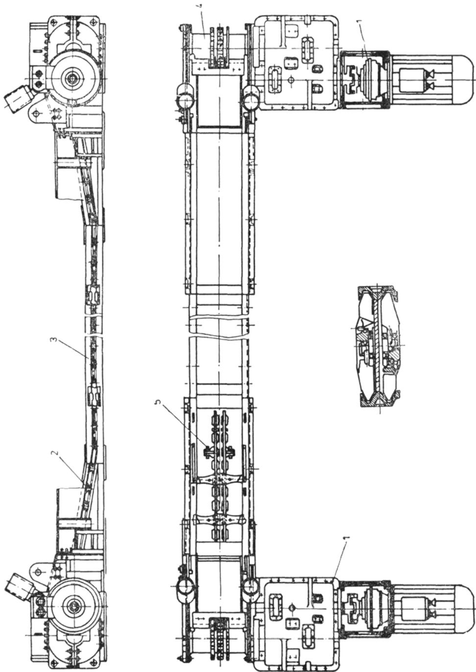
Fig. 1. TR-7A type push conveyor
