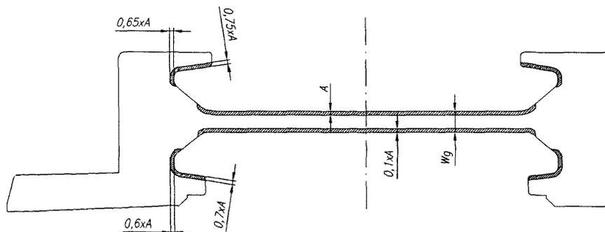
Fig. 9. Limits values of the slipping plate wear
