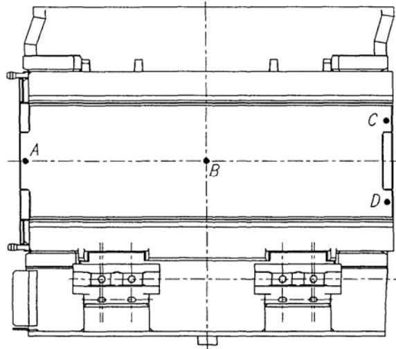
Fig. 8. Measurement points of the slipping plate thickness of Tagor conveyor
