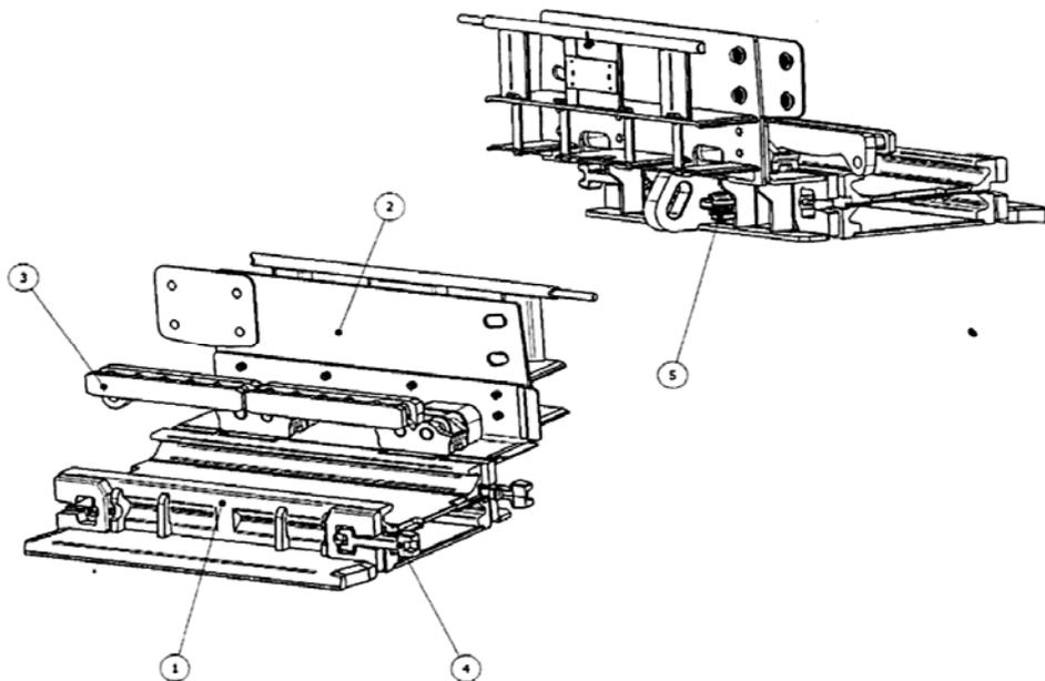
**Fig. 6.** Main raceway segment of TAGOR-260/750 type face conveyor:
