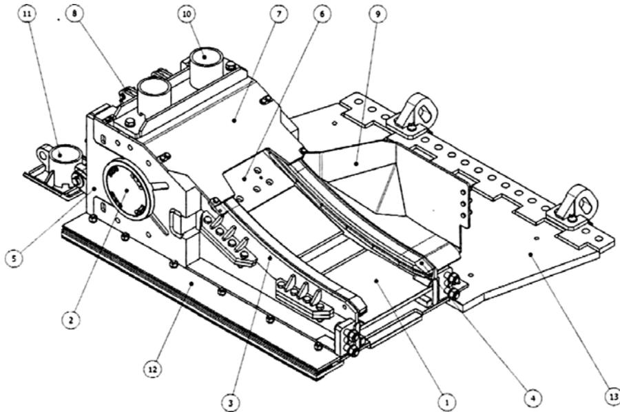
**Fig. 5.** Return station body of the TAGOR-260/750 type face conveyor:
