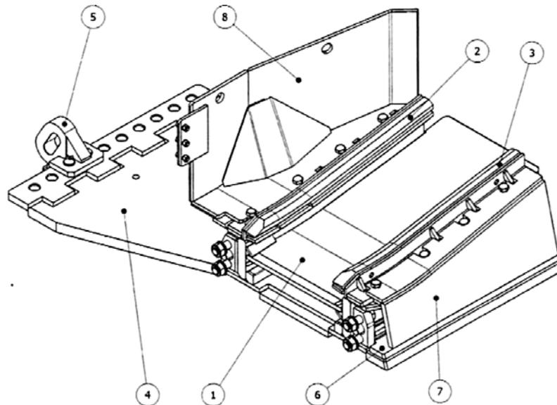
**Fig. 4.** The connection segment with lateral dumb of the TAGOR-260/750 type face conveyor:
