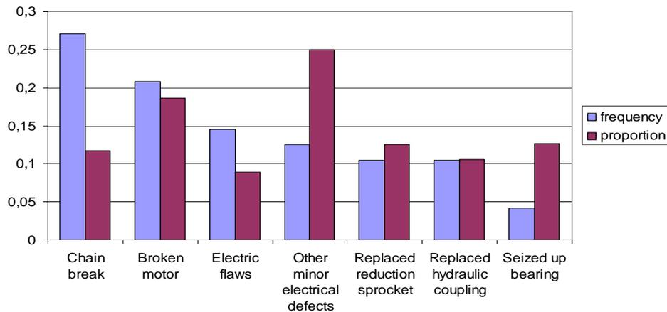
Fig. 7. Pareto diagram of TR-7A type conveyor failures
