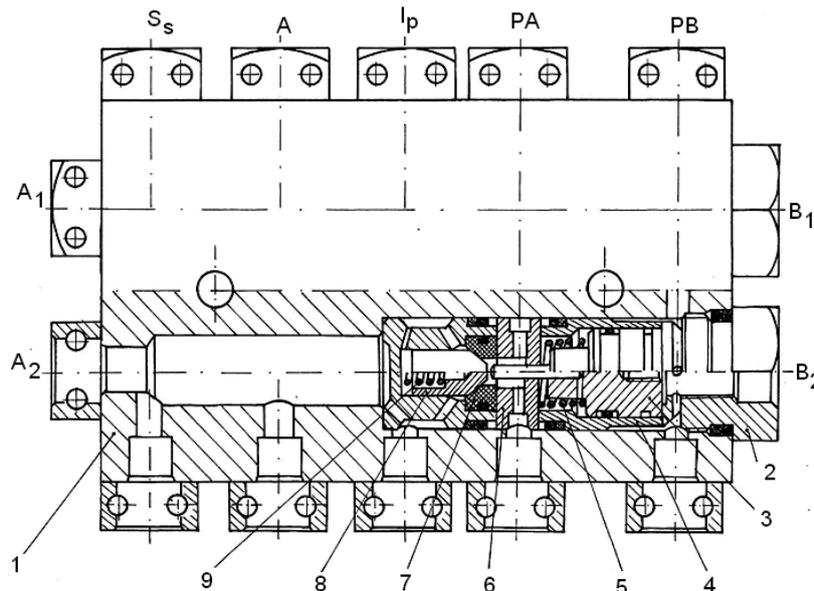
**Fig.8.** Double deblockable valve of direction:
