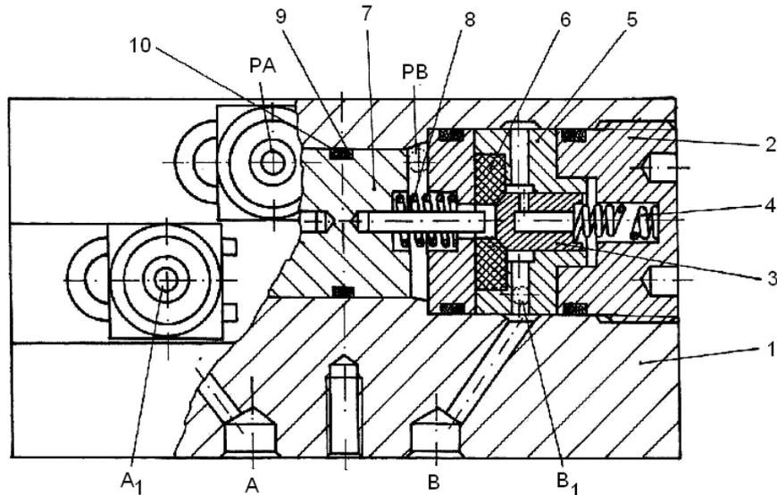
**Fig. 7.** Double deblockable valve of direction:
