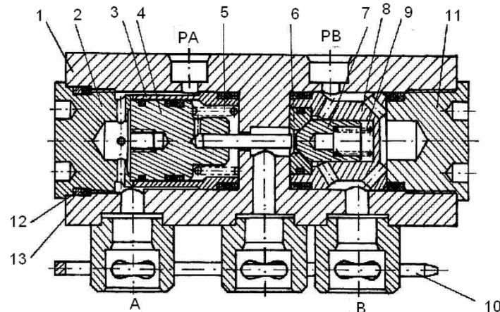
**Fig. 6.** Unblockable direction valve:
