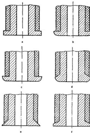
**Fig. 3.** Electrode-tools used to electrochemically deburr bore holes [12].
