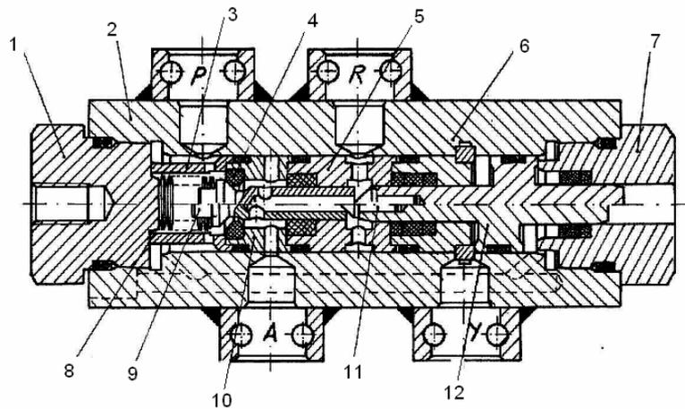
**Fig. 5.** Controlled direction valve normally open:
