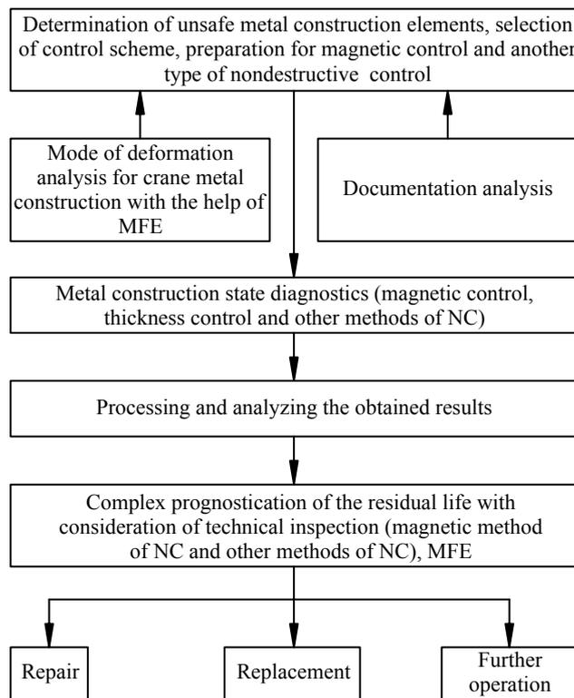
**Fig. 5.** Chart for prognosticating the remaining/residual life of bridge crane metal constructions with different element thickness with the help of magnetic (coercive metric) control method
