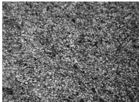
**Fig. 2.** Microstructure of 09Г2С steel sample (State Standard 19281-89), enlargement x 100, grain of point 9 (State Standard 5639-82)
