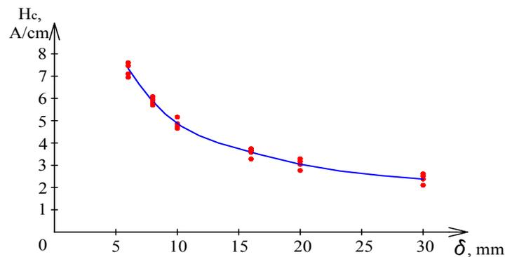
**Fig. 4.** Approximation of obtained results of coercive control in variable cross-section samples made of 10XCHД steel
