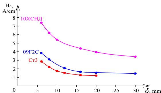
**Fig. 1.** - Dependence of coercive force value  $H_c$  (A/cm) on metal-roll thickness ( $d$ , mm) with grain-size of point 9 (State Standard 5639-82)
