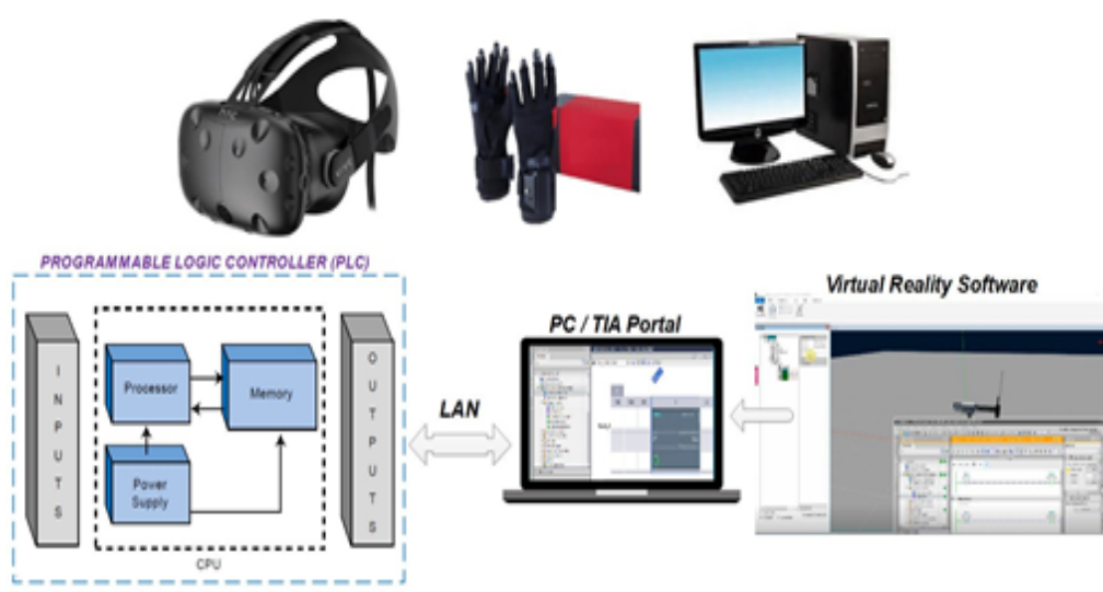
Fig. 2. Siemens PLC software communicating with virtual reality software
