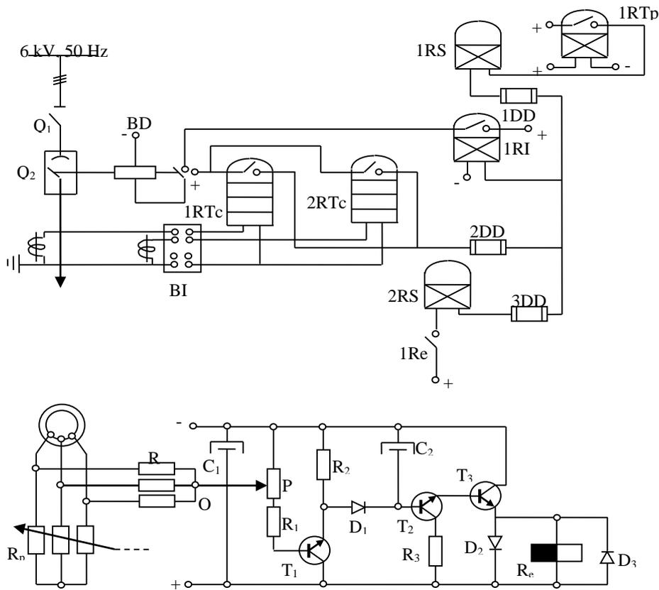
**Fig. 1** Operating principle of the protection relay
