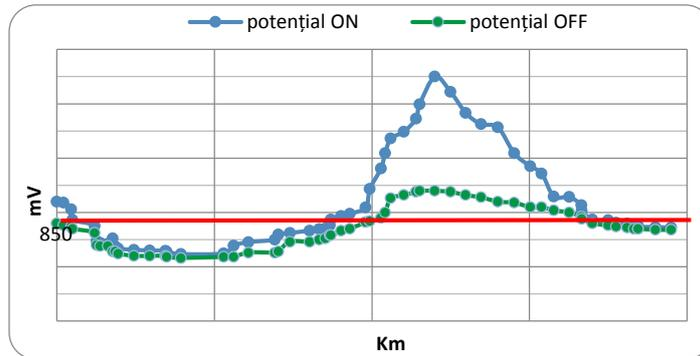
**Fig. 2** Potential diagram along the main pipeline
