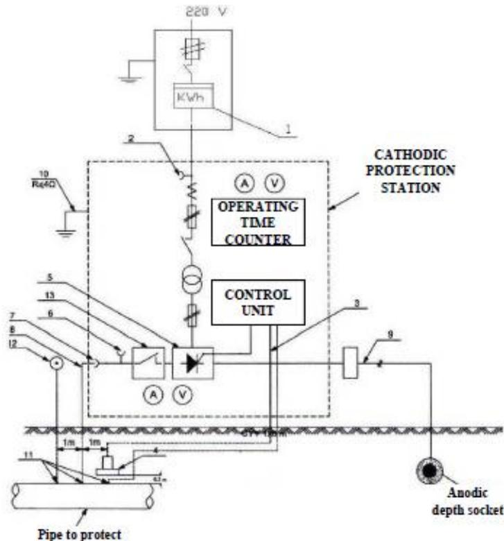
**Fig. 1** Schematic of a cathodic protection station
