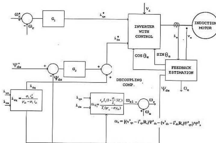
Fig. 4. Stator flux oriented direct vector control
