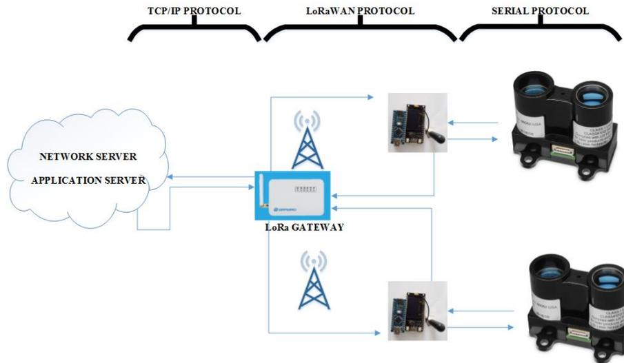
**Fig. 3.** The architecture of LoRa system
