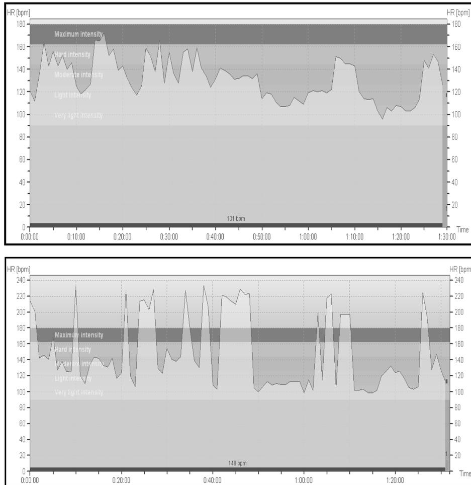
**Figure 4. The curve for the Heart Rate (HR) during a 90 minutes training program for two extreme cases of mine rescuers**
