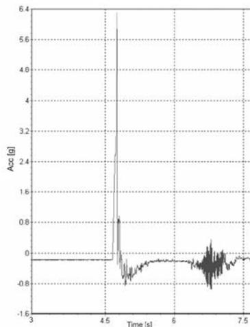
Figure 7. Variation of acceleration Acc1 as a function of time, during the collision process – loaded car
