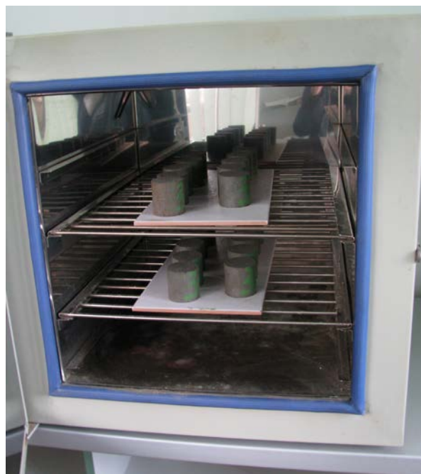
Fig. 3. Drying of the samples in an oven at 105 °C
