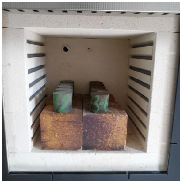
Fig. 4. Burning samples in a furnace at temperatures of 970 °C, 1000 °C, 1030 °C
