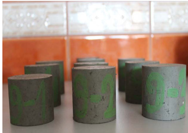
Fig. 2. Parts raw ceramic obtained by compression molding
