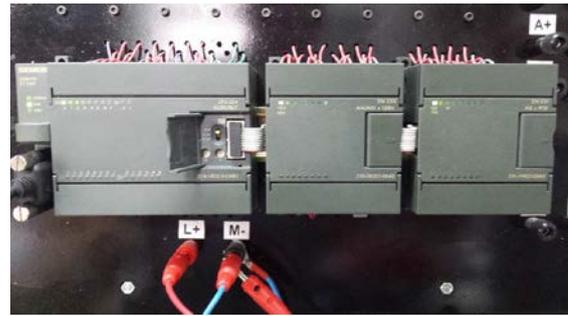
Fig.4. CPU 224 PLC and EM 235 and EM 231 RTD extension modules
