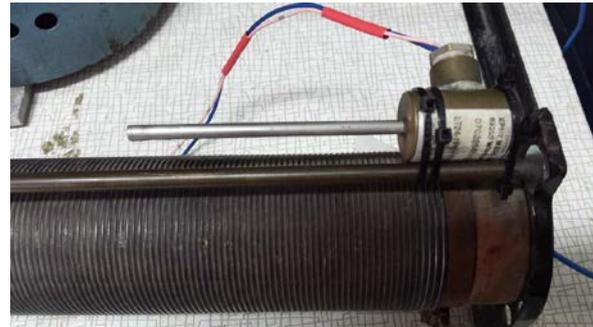
Fig.5. Pt 100 thermo-resistance used in experiments (connected on a power resistor)
