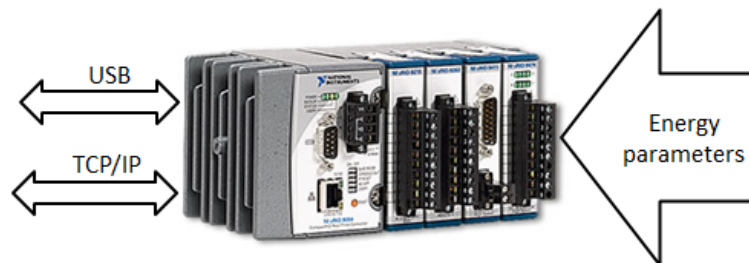
Fig. 12. The measurement structure
