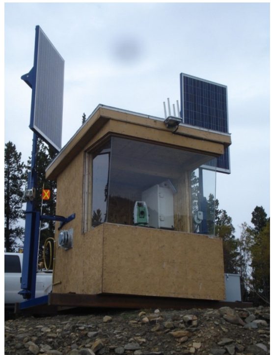
Figure 3. Total station monitoring inside weather protection shelters house
