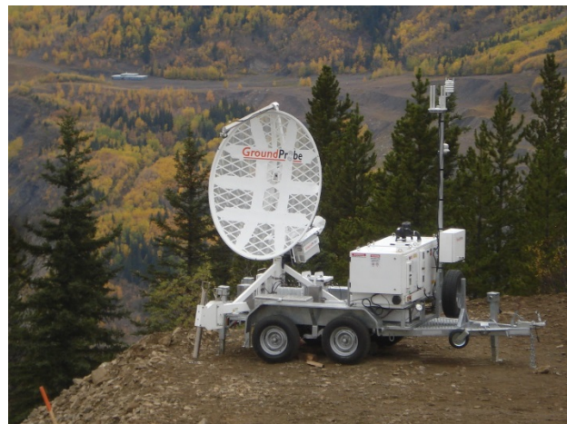
Figure 4. SSR-X radar monitoring system
