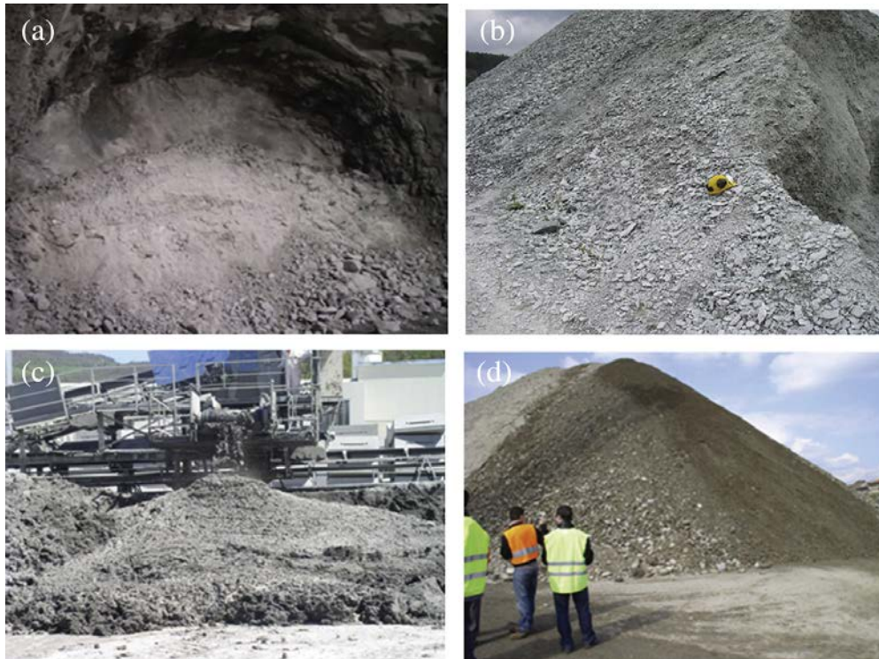
Figure 1. Examples of tunnel spoil types. (a) Granitic rock, Drilling and Blasting in large-section road tunnel (Omega Tunnel, Italy); (b) Granitic rock, full face TBM in small-section exploratory drift (Aica-Mules Tunnel, Italy); (c) Soft rock-hard soil, full face excavation and soil conditioning for large-section highway tunnel (Sparvo Tunnel, Italy); (d) Coarse soil, mechanised excavation for railway tunnel (Turin Railway “Passante”, Italy). (Oggeri et al., 2014)
