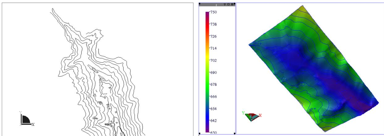
Fig. 8. Digitized level curves from aerial survey made in 1981 in Valea Arsului (left) and digital terrain model of Valea Arsului with sinking phenomenon (right)
