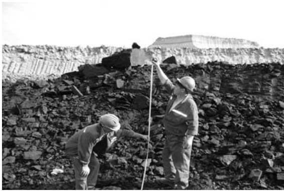
Figure 9 - Measuring the coal layer
